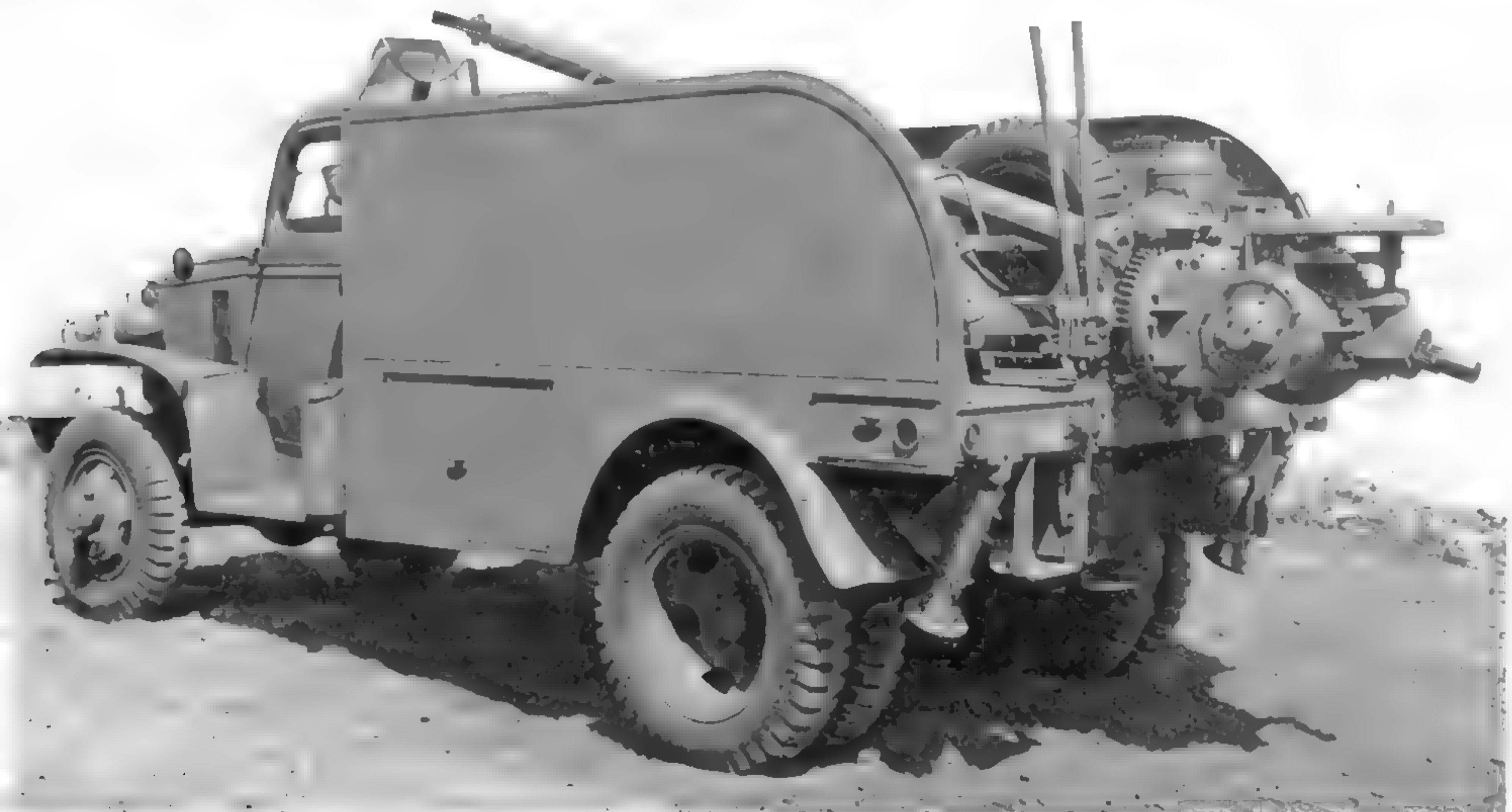
This left rear view of the K44 (G7163) pole setter shows the auger, in the lowered transport position, and its two long operating levers. Also visible are the two stabilizer jacks, in their raised transport position. Near the spare tire is the drinking water cask found on Signal Corps vehicles. (U.S. Army photo)
